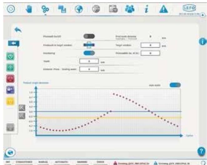
▲ The print mark detection is one of the default features that are already stored in the machine control system that reduces the machine operator's programming effort
