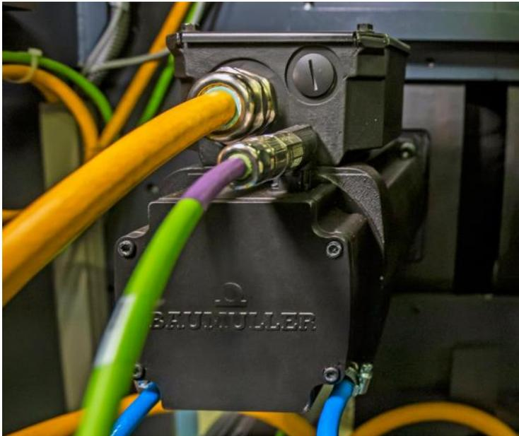
**Figure 3:** DSD2 servomotors are dynamic and slim in design. They are water-cooled in the film feed, which enables high performance in a very small installation space at the same time
